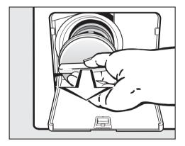
■ Unscrew the drain filter completely.
